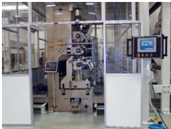
Cartridge coaters can be removed for fast and easy cleanup of laminating adhesives.
