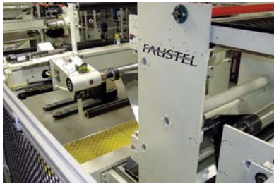
Dual-direction flying fly splicers on unwinds are designed to unwind and splice thin aluminum foils at full speed.
