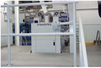
Flexographic printer features sleeved plate cylinders, servo-motor drive and the ability to print either side of the web prior to coating and laminating.
