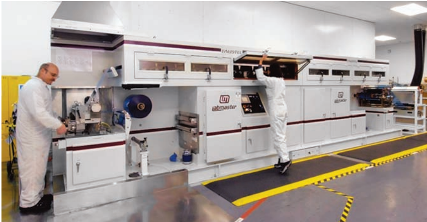
The Faustel LabMaster line is described as "Plug & Play"—a pre-engineered pilot coater/laminator designed for R&D and narrow-web production coating/laminating.
