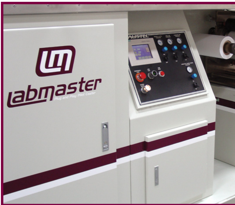
Operator's control station and storage compartments
